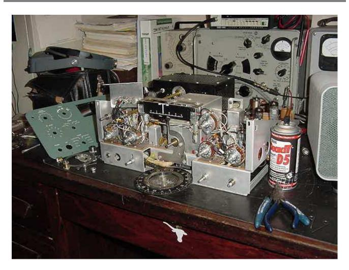
The "SB-101/SB-102 specific" information for this site is still being developed. They are pretty rugged units and I've found some weak tubes, a few tubes with grid emissions, the usual requirement for alignment per the manual, and slipping tuning dials needing adjustment. And yes, they are a poor (but smart) man's Collins.
